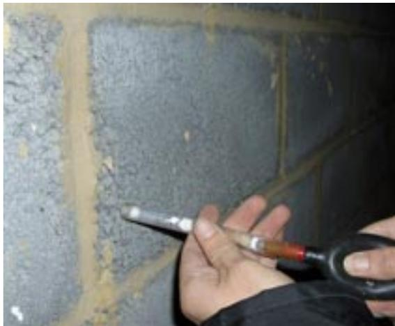
Figure 4 Air permeability through gaps in a blockwork wall.
