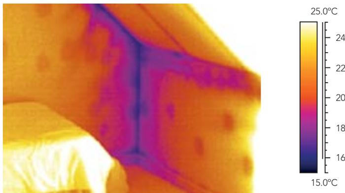
**Figure 6** The effects of cold air behind dry lining attributed to air leakage.
