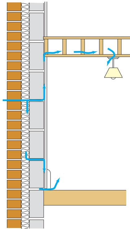
Figure 5 Air leakage through gaps and missing mortar joints in a blockwork wall.
